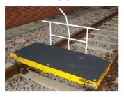
All hand trolleys used on Network Rail managed Infrastructure must be fitted with operational brakes (a "fail safe" braking system") and the correct brake handle must be used when operating the hand trolley.
